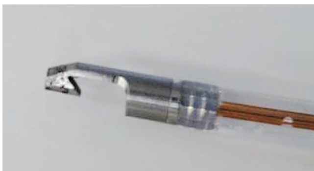
Fig. 3: "Hot tip" device. Vessel coagulation is possible by laser irradiation to the tip of the device and submucosal dissection is possible by using hooking part.
