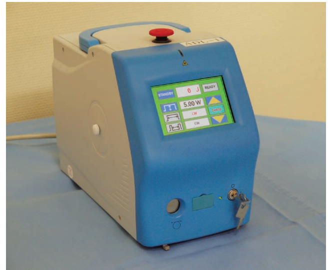
Fig. 2: The diode laser device as developed by Asuka Co. Japan. Maximum output 8 W with pulse preset at 0.5 s. Note the dimensions of the system were much smaller than the diode laser pumped Nd; YAG laser device used in 2005.
